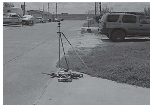
A post-pointed GCP - Crigth angle intersection of two contrasting features
