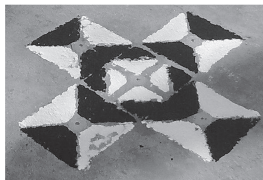
Improperly designed target - poor definition of dot size, repetitive pattern, less contrasting
