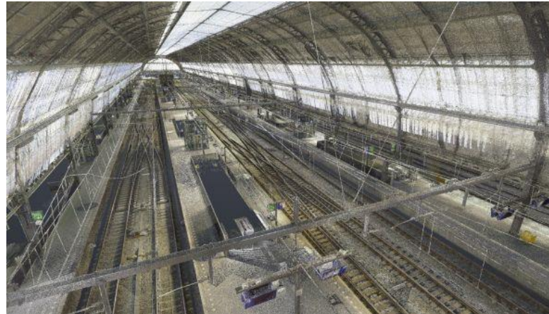
Lidar point cloud of Amsterdam Centraal Station.
