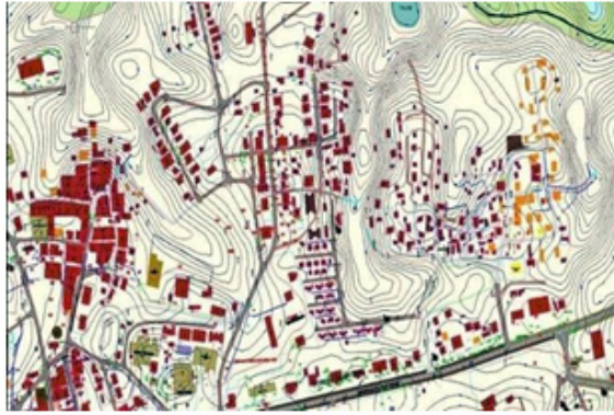
Figure 4: Contour Map generated from LiDAR data which enables better understanding of the catchment area for the administrators
