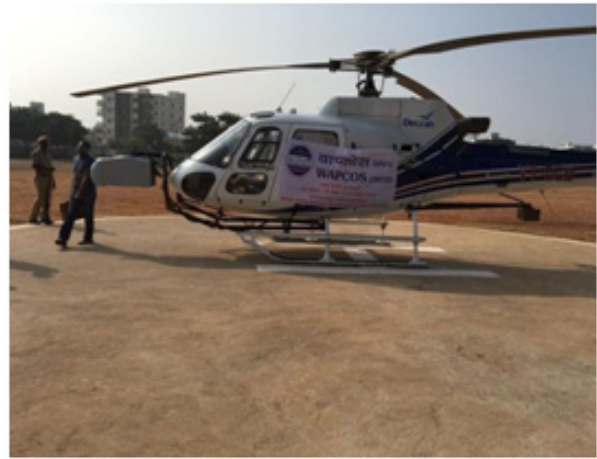
Figure 5: Helicopter ready for surveying with sensors fitted
